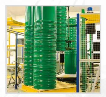
Up to 104 empty conical drums can be nested and stored per pallet.
